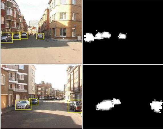
Figure 7. (left) Successful car detections. (right) Corresponding car segmentation masks fed back to the SfM module.
