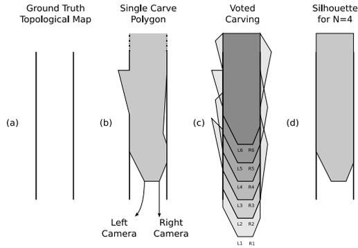
Figure 3. (a) Example of a ground truth topological map. (b) Polygon extracted for a single stereo set. (c) Voted carving. (d) Resulting topological map from silhouette extraction.
