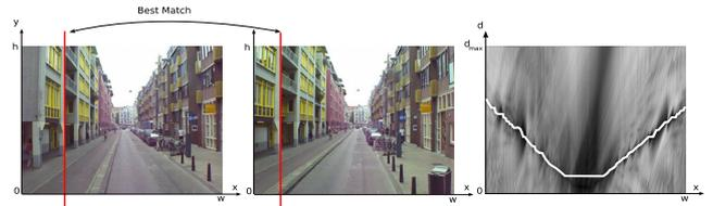
Figure 2. Left and middle: Rectified stereo pair with example of a best match, based on an aggregated similarity measure along the vertical image direction. Right: Computed similarity map with optimal path resulting from dynamic programming (white line).
