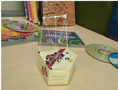
Figure 1: A plane (top surface of packaging) accidentally picks up interest points in the background. Therefore we split the interest point clusters (coloured dots) using the mean and standard deviation of edges of a Delaunay graph (white edges).
