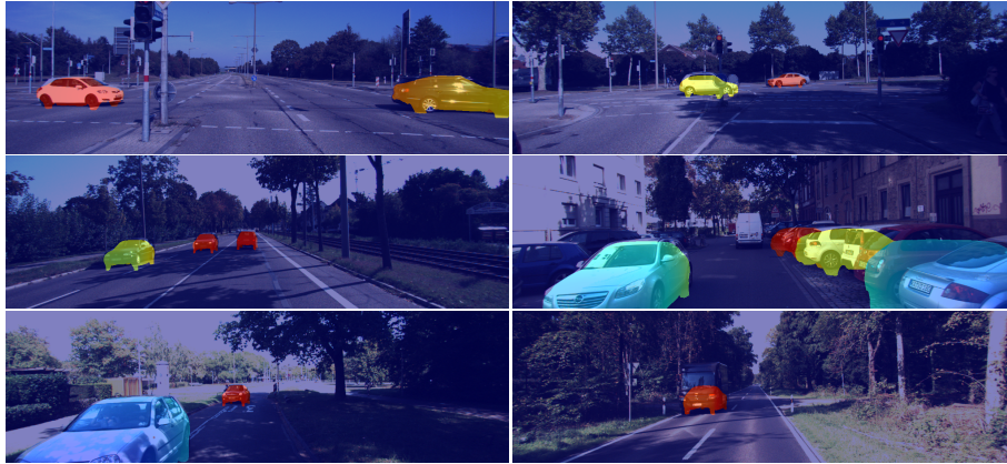
Fig. 6. Example depth reconstruction and segmentation results for libELAS depth input. Disparity encoded from small (red) to large (blue) values. Right column shows problematic examples for our method. See text for a detailed discussion.
