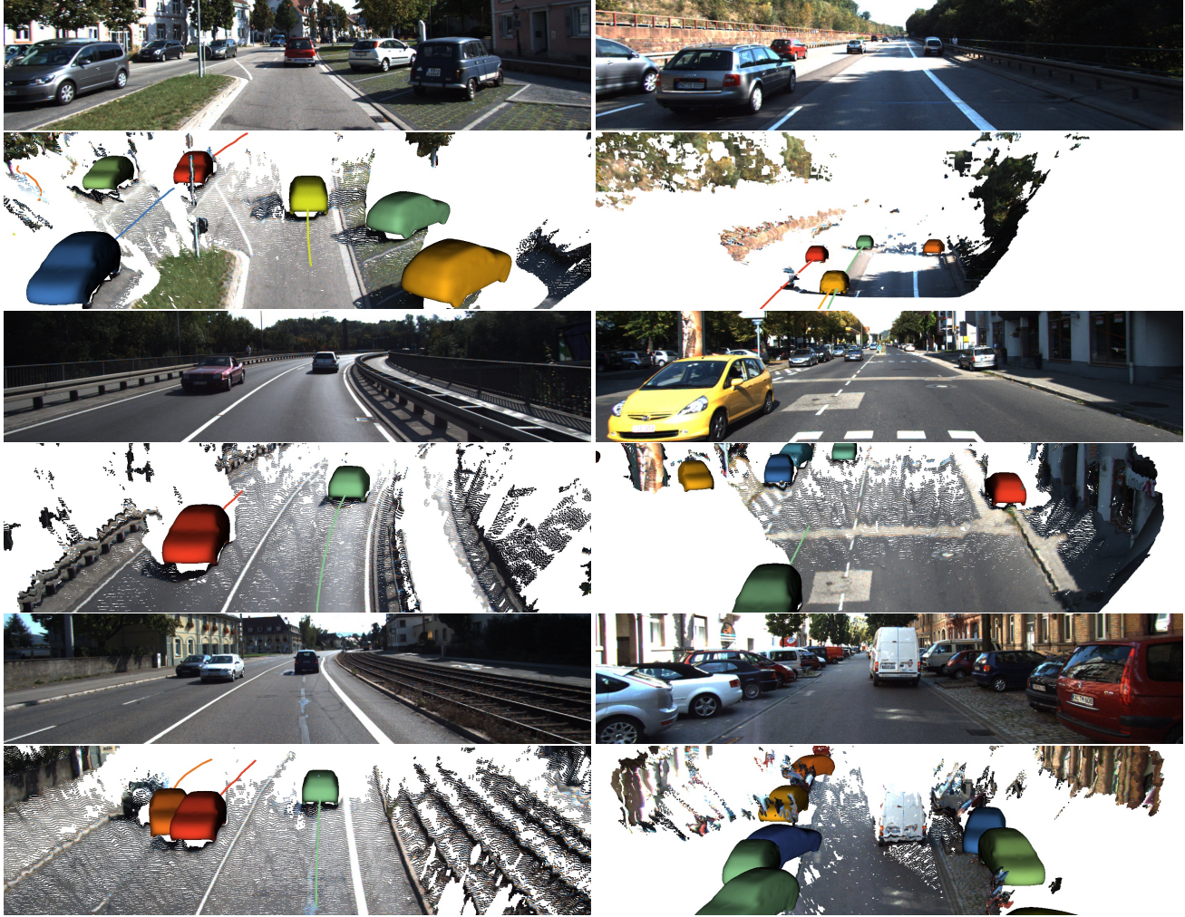
Figure 10. Qualitative Results. First two rows show exemplary good results of our method. Last Row: Failure cases. Left: Initial tracklets of two vehicles are merged during the optimization due to noisy 3D detections. Right: Wrong initial detections and tracking associations that cannot be corrected by our method.
