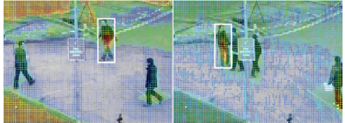
Fig. 5: The classifier response (heat map) visualized for one tracking target (white). As the classifier is adapted continuously, it becomes more discriminative (right: 20 frames later).
