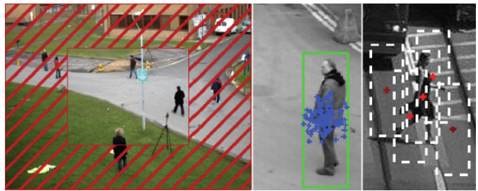
Fig. 3: The initialization and termination region for a typical surveillance scenario (left). The initial particles are drawn from a normal distribution centered at the detection (middle). The weight of each particle is determined by evaluating the respective image patch (right).
