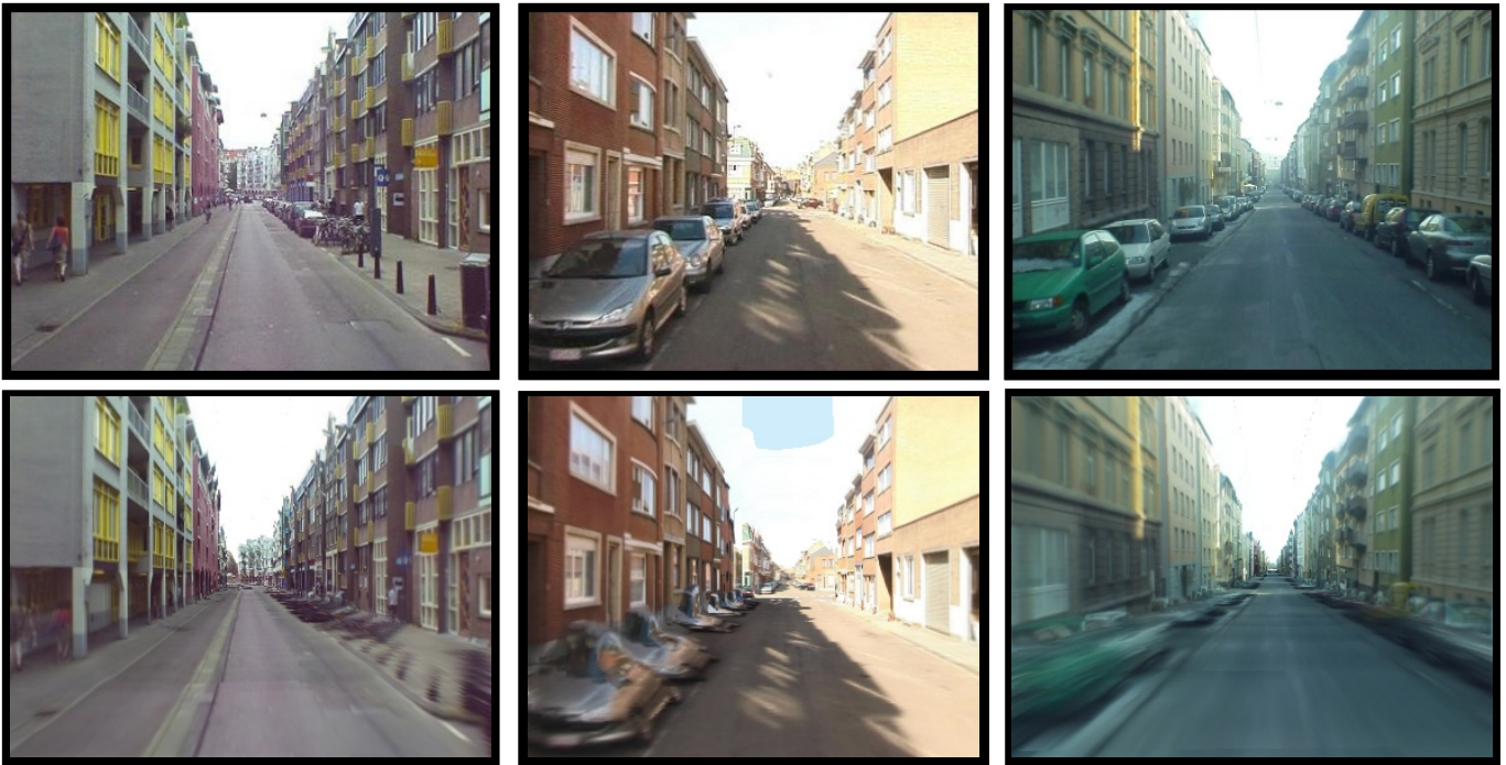
Fig. 11. (top) Undistorted images, taken directly from the video stream; (bottom) rendering of the reconstructed models from the same point of view.
