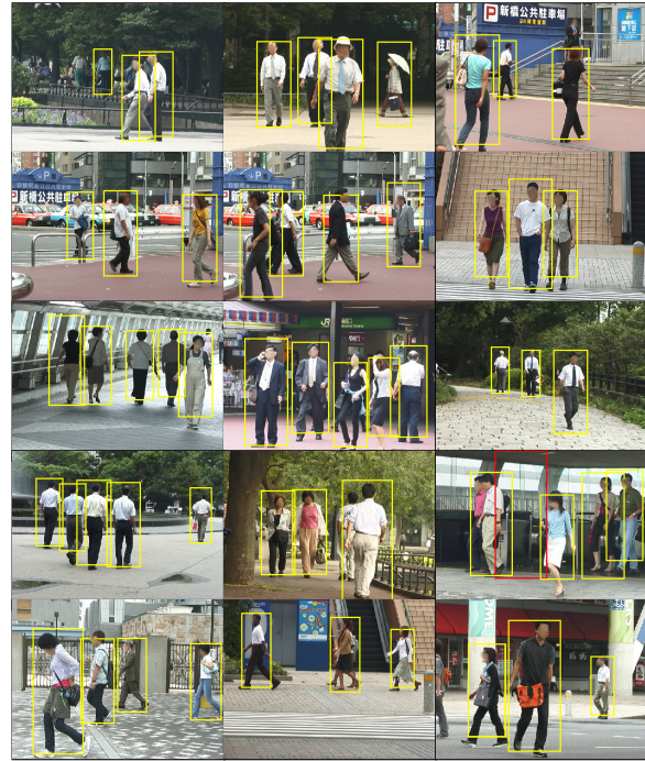
Figure 9. Example detections (in yellow) and false positives (in red) on testset B at the EER.
