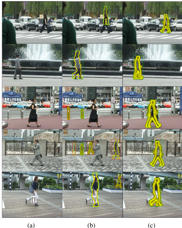
Figure 6. Articulation estimates containing typical failure cases for Chamfer verification (silhouettes and shape clusters drawn in yellow) – (a) test image, (b) Chamfer verification hypothesis, (c) 4D-ISM articulation estimate
