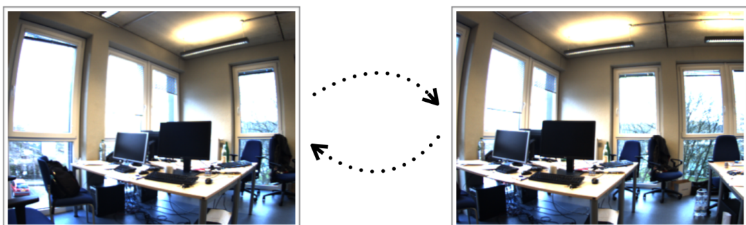
Figure 3.8: The example of two images that are not exactly the same, but should be matched as similar to perform the loop closure.
